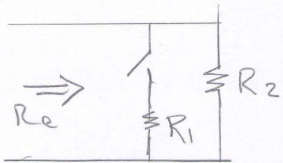
During on state the input resistance =  $R_1 \parallel R_2$
